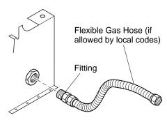
Figure 10 - Attaching Flexible Gas Hose to Heater
